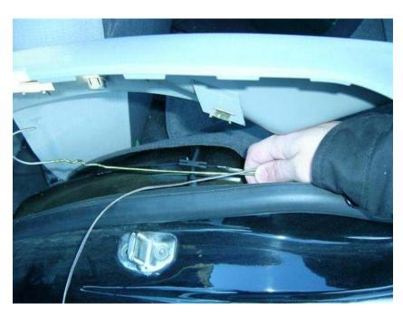
Take the hanger and push the wire all the way to the back of the car. Open the CD changer door, and the lamp access door. It will be above the tail light. It was kinda a pain to grab the wire, but I was able to. A helper might be good here to operate the hanger while you try to grab the wire. I suppose you could just try to push the wire back without using the hanger or fish tape... but I think it made life easier.
