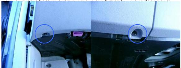
This also lets the plastic piece above the pedals loose. If you pull it straight forward, it comes off. Note the tabs on the front, and the white catches attached to the front of the car.
