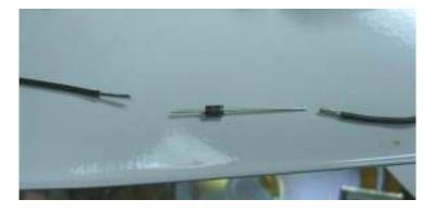
I found that made it easier to solder the diode on, because the solder was already on the wires.
