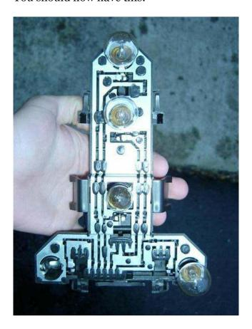
The top bulb is the normal brake light. Next is the turn signal, then the marker light. The one on the right is the reverse light. The empty socket is for the rear fog. Install a bulb there. This is mirrored on the passenger side of the car.
