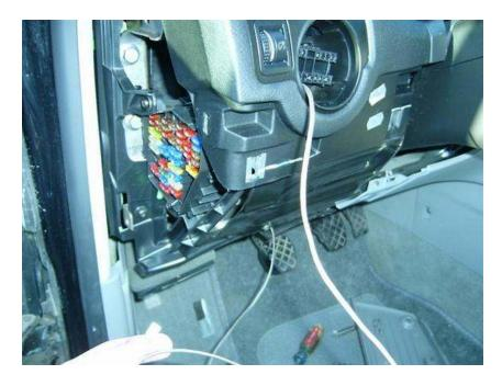
A word of caution here. The wire is going past the power center of the car. I would put a piece of tape over the female connecter: don't want it to short anything out
