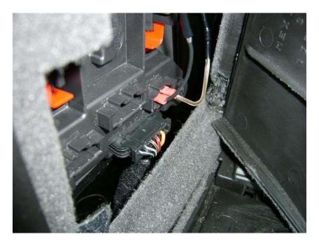
Woot! Driver's side is done! The passenger side is easier. Open the access door on the passenger side. Squeeze the clips again. The sockets are easier to get out on this side. Install a bulb in the empty socket. Run the jumper (the one without a diode.. the only one left hopefully) from the brake light pin to the rear fog pin. NOTE, this will be opposite of the way it was on the drivers side.
