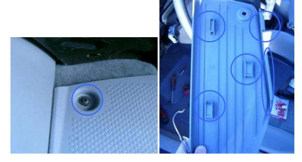
It was a real pain to get that thing off. With the screw out, it slides up and the 3 tabs on the 'face' disengage, but there are also 2 tabs that hold the pedal to the trim along the side of the car. You can see them in that pic. Just go slow, and don't try this when the plastic is cold and brittle I guess. For reference, here is what's under the dead pedal:
